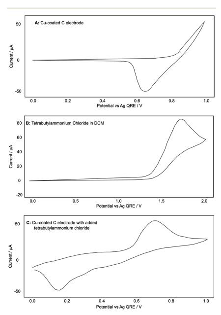
Fig. 8 (A–C): representative CV plots examining the effect of chloride on the release of copper from a Cu-coated glassy carbon electrode recorded in 0.1 M  $\rm Bu_4NPF_6/DCM$  with a Ag QRE and a Pt CE.
