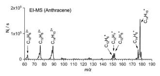
Fig. 1 EI-MS spectrum of anthracene. The arrows denote which cations were selected for further screening.
