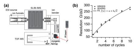
Fig. 1 (a) Schematic overview of the instrument combining ultra-high resolution SLIM IMS techniques with messenger-tagging IR spectroscopy. (b) IMS resolution of the new instrument as a function of SLIM cycles (IMS path length) determined by monitoring the peak widths and positions of two isomeric MS standard peptides GRGDS and SDGRG in their doubly protonated forms.
