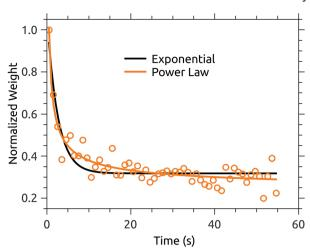
Fig. 7 Normalized projection (or weight) of the first principal component of the 60 s action spectrum time series of coronene cations in DESIREE. A power-law fit better represents the cooling curve than a single exponential decay.
