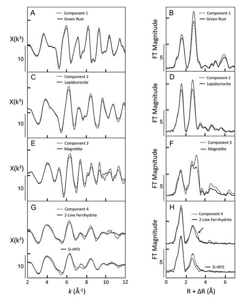
Fig. 3 Comparison of ITFA-derived components and Fe K-edge EXAFS spectra of Fe-bearing reference materials. The EXAFS spectra are given in the left panel and the corresponding Fourier transforms are shown in the right panel. The dotted black lines represent the components and the solid black lines represent measured reference spectra. The arrow in H highlights features in the Fourier-transformed EXAFS spectrum of 2-line ferrihydrite that arise from corner-sharing Fe-Fe bonds.
