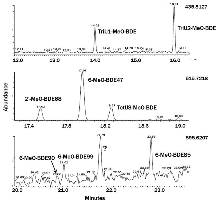
Fig. 2 GC-HRMS of tribromo-, tetrabromo- and pentabromo-MeO-BDEs (upper, middle and lower, respectively) in *Fucus radicans* from the Bothnian Sea. Monitored ions are given at the upper right of each panel. TriU1-MeO-BDE, TriU2-MeO-BDE and TetU3-MeO-BDE have unknown bromine substituent positions. The marked peak (?) at 21.78 min has not been identified, but does not have the correct ion ratios for a pentabromo-MeO-BDE.
