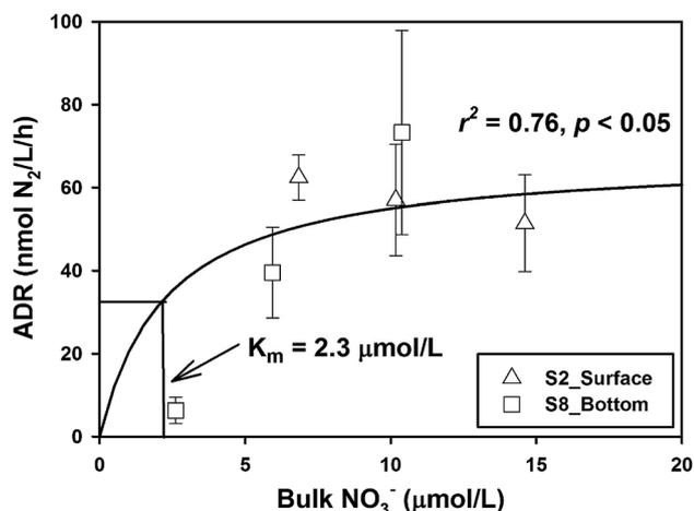
Fig. 2 Response of apparent denitrification rate (ADR) with manipulated NO<sub>3</sub><sup>-</sup> concentration at Stations S2 and S8. The solid line is fitted according to the Michaelis–Menten kinetics.  $K_m$  represents the half-saturation constant of NO<sub>3</sub><sup>-</sup> demand.
