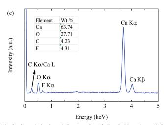
Fig. 3 Characterization of Ca deposits. (a) The PXRD pattern of Ca deposits. (b) The SEM image of the deposits; the scale bar is 250  $\mu m$ . (c) The EDX spectrum within the white squared area.
