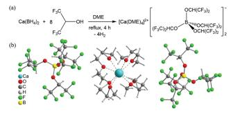
Fig. 1 Synthesis (a) and X-ray single-crystal structure (b) of Ca[B(hfip)<sub>4</sub>]<sub>2</sub>.
