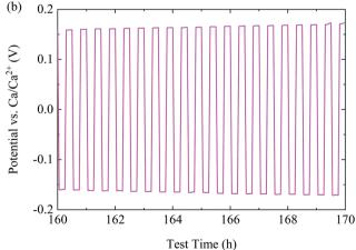
Fig. 4 (a) The cycling performance of the CaBhfip/DME electrolyte at various current densities. (b) A typical voltage profile at a current density of  $0.2 \text{ mA cm}^{-2}$
