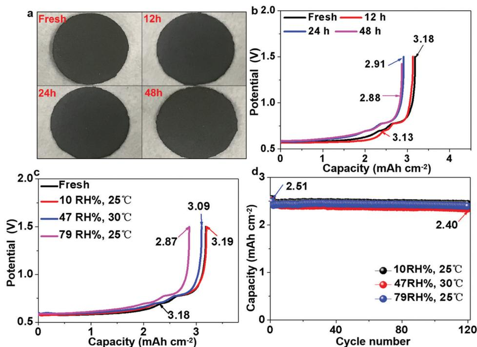
Fig. 6 Air stability analysis of Li<sub>x</sub>Sn foil. (a) Visual images of Li<sub>x</sub>Sn foils exposed to ambient air for different periods. (b) Lithium inventories of Li<sub>x</sub>Sn electrodes exposed to ambient air for different periods. (c) Lithium inventories of Li<sub>x</sub>Sn electrodes exposed to various humidity for 12 h. (d) Cycle performance of Li<sub>x</sub>Sn electrodes exposed to different humidity for 12 h in full-cell cycling.
