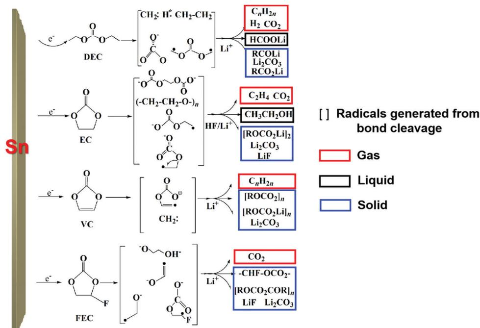
Fig. 4 The possible pathways of carbonate-based electrolyte decomposition on the Sn foil surface.
