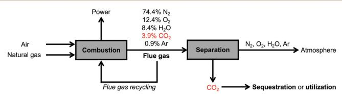
Fig. 2 Schematic of a natural gas-fired power plant with post-combustion CO2 capture, including optional flue gas recycling to increase the concentration of  $CO_2$  in the flue gas up to  $\sim 8\%$ .
