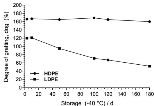
**Fig. 1** Degree of grafting (dog) of poly(VBC)-grafted membranes made from e-beamed LDPE and HDPE films that were stored (pre-grafted) at -40 °C for increasing periods of time. The dog (%) was calculated as:  $\text{dog} = 100 \times (m_g - m_i)/m_i$  (where  $m_i$  was the mass of the e-beamed pre-grafted film and  $m_g$  was the mass of the (pre-aminated) VBC-grafted membrane).<sup>7</sup>
