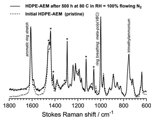
**Fig. 3** The Raman spectra of the HDPE-AEM before and after the 500 h test presented in Fig. 2. A ThermoFisher DRX Raman microscope (532 nm laser) was used. Key diagnostic peaks<sup>4</sup> are labelled; \* = HDPE-derived peaks. The spectra were normalised to the trimethylammonium peak at 753 cm<sup>-1</sup> to aid visual comparison.
