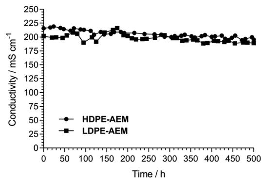
**Fig. 2** Changes in OH<sup>-</sup> conductivity of the RG-AEMs when placed in a flowing relative humidity RH = 100% N<sub>2</sub> atmosphere at 80 °C for 500 h. Method discussed in detail in ref. 4 (where the LDPE-AEM data was first reported).
