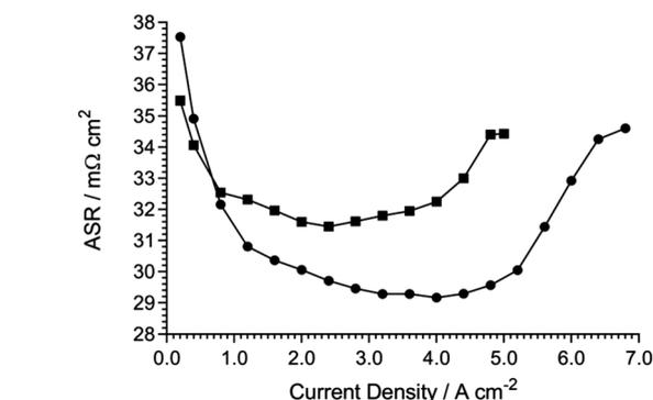
Fig. 6 Comparison of HDPE-AEM-containing  $\text{H}_2/\text{O}_2$  AEMFC performances at  $80^\circ\text{C}$  with cathodes containing a Pt/C catalyst (40 wt% Pt,  $0.4 \text{ mg cm}^{-2}$  Pt loading) and a Ag/C catalyst (40 wt% Ag,  $0.85 \text{ mg cm}^{-2}$  Ag loading). All other MEA and cell test parameters as in Fig. 4.<sup>4</sup> ASRs were measured using the 850E tester's internal current interrupt method.
