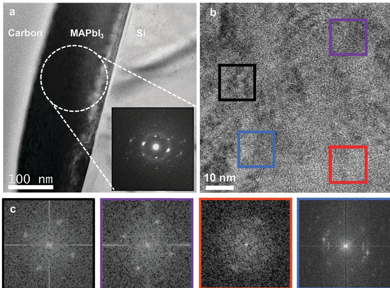
Fig. 4 TEM electron diffraction analysis of MAPbI<sub>3</sub> perovskite grains. (a) Cross-section image of single perovskite grain on Si(100) substrate and selected area electron diffraction (SAED) pattern collected from the region indicated (inset). (b) Higher-magnification TEM and (c) fast Fourier transform (FFT) patterns generated across different regions of the grain shown in (b).
