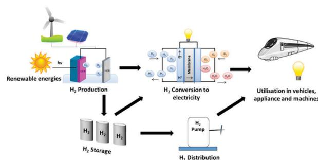
Fig. 1 Schematic of a simple hydrogen economy concept.
