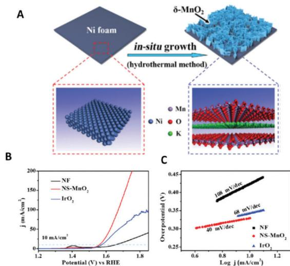
Fig. 9 Schematic showing the *in situ* growth of ultrathin  $\delta$ -MnO<sub>2</sub> nanosheets on an Ni foam (NS-MnO<sub>2</sub>). (A) Linear sweep voltammometry (LSV) curves for OER at a scan rate of 5 mV s<sup>-1</sup>. (B) Tafel plots for OER. (C) LSV curves for HER at 5 mV s<sup>-1</sup>. (Reproduced with permission (ref. 104) Copyright Wiley and Sons (2017).)
