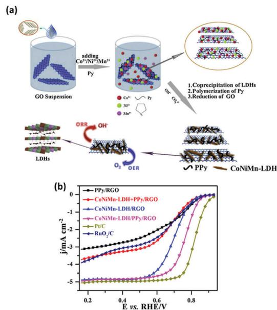
Fig. 18 (a) Schematic illustration of fabrication process towards CoNiMn-LDH/PPy/RGO for oxygen reduction reaction and (b) LSV curves of the four samples, 20 wt% Pt/C, and 20 wt%  $\text{RuO}_2/\text{C}$  catalyst at 1600 rpm in  $\text{O}_2$ -saturated 0.1 M KOH. (Reproduced with permission (ref. 125) Copyright Elsevier (2017).)
