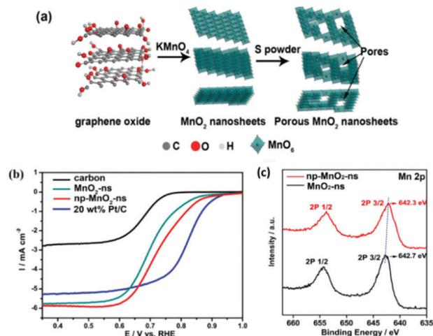
Fig. 16 (a) Schematic diagram for the synthesis of np-MnO<sub>2</sub>-ns and (b) ORR performance of carbon, MnO<sub>2</sub>-ns, np-MnO<sub>2</sub>-ns, and 20 wt% Pt/C in O<sub>2</sub>-saturated 0.1 M KOH aqueous solution at room temperature, LSV measured at 5 mV s<sup>-1</sup> and 1600 rpm and (c) XPS curves for the MnO<sub>2</sub>-ns and np-MnO<sub>2</sub>-ns materials. (Reproduced with permission (ref. 74) Copyright Wiley and Sons (2018).)
