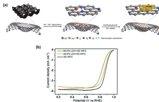
Fig. 17 (a) Schematic illustration of the synthesis of nNiFe LDH/3D MPC and (b) ORR LSV curves for nNiFe LDH/3D MPC, bNiFe LDH + 3D MPC and 3D MPC in 0.1 M KOH at a scan rate of 5 mV s<sup>-1</sup> with a rotation speed of 900 rpm. (Reproduced with permission (ref. 123) Copyright Royal Society of Chemistry (2018).)
