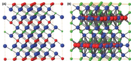
Fig. 4 The structural models of layered oxides containing alkali metal and transition metal. The structure of LiCoO<sub>2</sub> (A) and (B) mineral birnessite (K<sub>0.48</sub>Mn<sub>1.97</sub>O<sub>5.18</sub>) based on layers of alkali metals and oxygen octahedrally coordinated transition metal layer.
