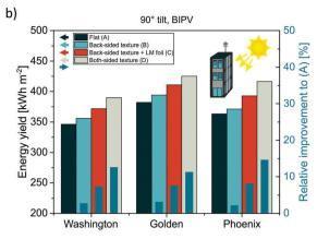
Fig. 6 Simulated yearly energy yield for different device designs (A), (B), (C), and (D) for (a) 30° and (b) 90° solar cell orientation/inclination and relative improvement to design (A) (right y-axis). Three different locations, Washington DC, Golden and Phoenix are compared.
