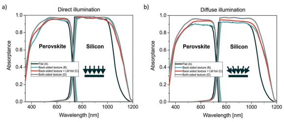
Fig. 5 (a) Simulated absorption spectra for the device designs (A), (B), (C) and (D) and perovskite thickness 1000 nm where direct illumination is considered. (b) Simulated absorption spectra for the device designs (A), (B), (C) and (D) and perovskite thickness 1000 nm where diffuse illumination is considered
