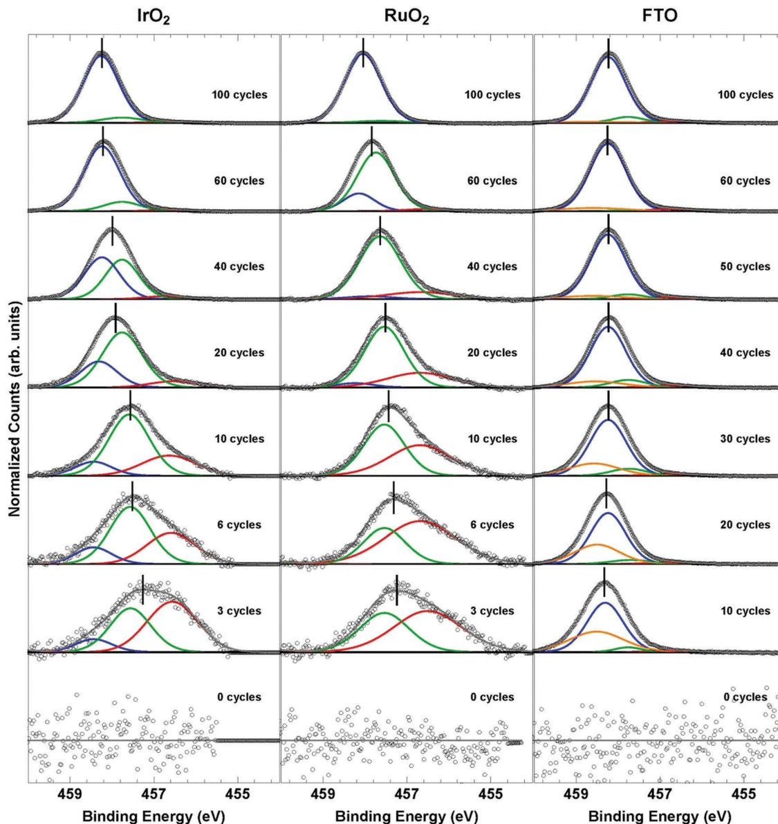
Fig. 4 X-ray photoelectron spectroscopy of the Ti  $2p_{3/2}$  region for  $\text{IrO}_2$ ,  $\text{RuO}_2$ , and FTO catalysts with varying  $\text{TiO}_2$  thicknesses. Bulk  $\text{TiO}_2$  is shown as the blue peak in each spectrum. The slightly and highly reduced Ti peaks are shown in green and red, respectively, and the most highly oxidized Ti peak is shown in orange.
