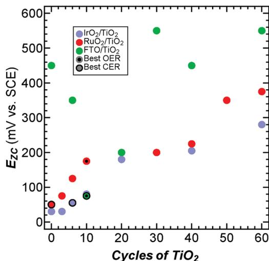
Fig. 3  $E_{ZC}$  of  $\text{IrO}_2$  (blue),  $\text{RuO}_2$  (red), and FTO (green) anodes coated with various ALD cycles of  $\text{TiO}_2$ . Black dots and circles with black borders indicate the catalysts with the highest specific activity for each catalyst for the OER and CER, respectively.
