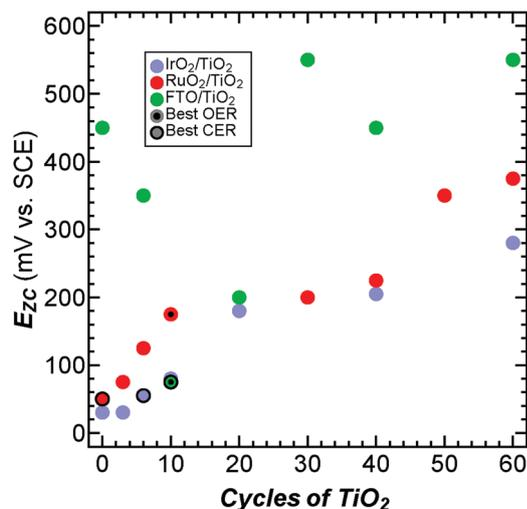
Fig. 3  $E_{ZC}$  of IrO<sub>2</sub> (blue), RuO<sub>2</sub> (red), and FTO (green) anodes coated with various ALD cycles of TiO<sub>2</sub>. Black dots and circles with black borders indicate the catalysts with the highest specific activity for each catalyst for the OER and CER, respectively.
