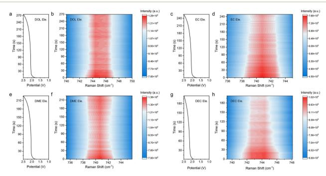
Fig. 6 In situ Raman measurement of the electrolytes near the surface of the LTO anode in LTO||LFP batteries during the fast charging process. Galvanostatic charging voltage curves of LTO||LFP full cells at 10C in (a) DOL Ele., (c) EC Ele., (e) DME Ele., and (g) DEC Ele. Corresponding variations of S-N-S stretching vibrations in (b) DOL Ele., (d) EC Ele., (f) DME Ele., and (h) DEC Ele.
