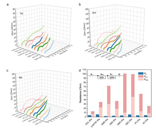
Fig. 5 EIS analysis of LTO||LFP batteries with different electrolytes. (a) 1st, (b) 3rd and (c) 5th cycles. (d) Resistance of bulk (R<sub>b</sub>), resistance of the SEI ( $R_{SEI}$ ) and resistance of the charge transfer reaction ( $R_{ct}$ ) calculated by fitting the data with the inserted equivalent circuit model. The batteries were charged and discharged at 1C, and the EIS were obtained during the charging platform of the batteries.
