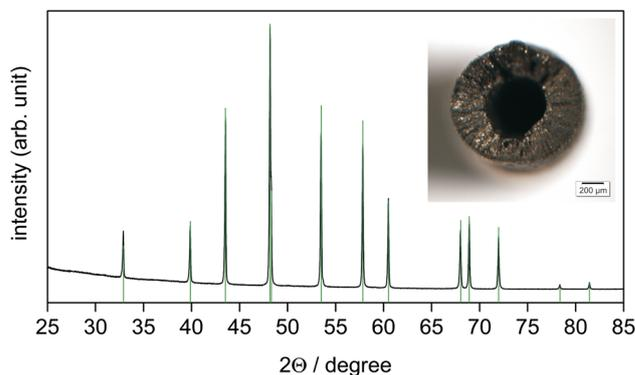
Fig. 2 The X-ray powder diffraction pattern ( $\text{CoK}_{\alpha}$  radiation) of the reaction product obtained at 800 °C after 30 min,  $p(\text{BBr}_3) = 94$  mbar,  $p(\text{Ar}) = 1.9$  mbar. Reflection positions (green ticks) and the relative intensities of  $\text{CoB}$  were calculated using the refined lattice parameters (Table 1) and the atomic coordinates according to ref. 33, respectively. The inset shows the reaction product as a hollow tube with a diameter of 1.2 mm.
