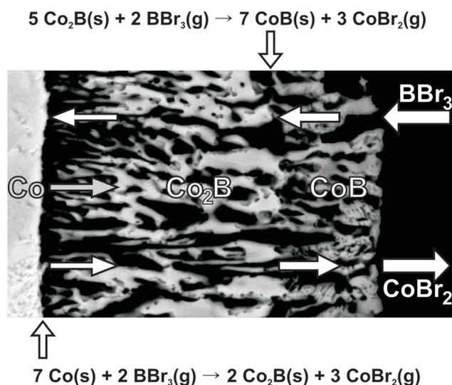
**Fig. 9** Scheme of the reaction between Co and BBr<sub>3</sub> (g).
