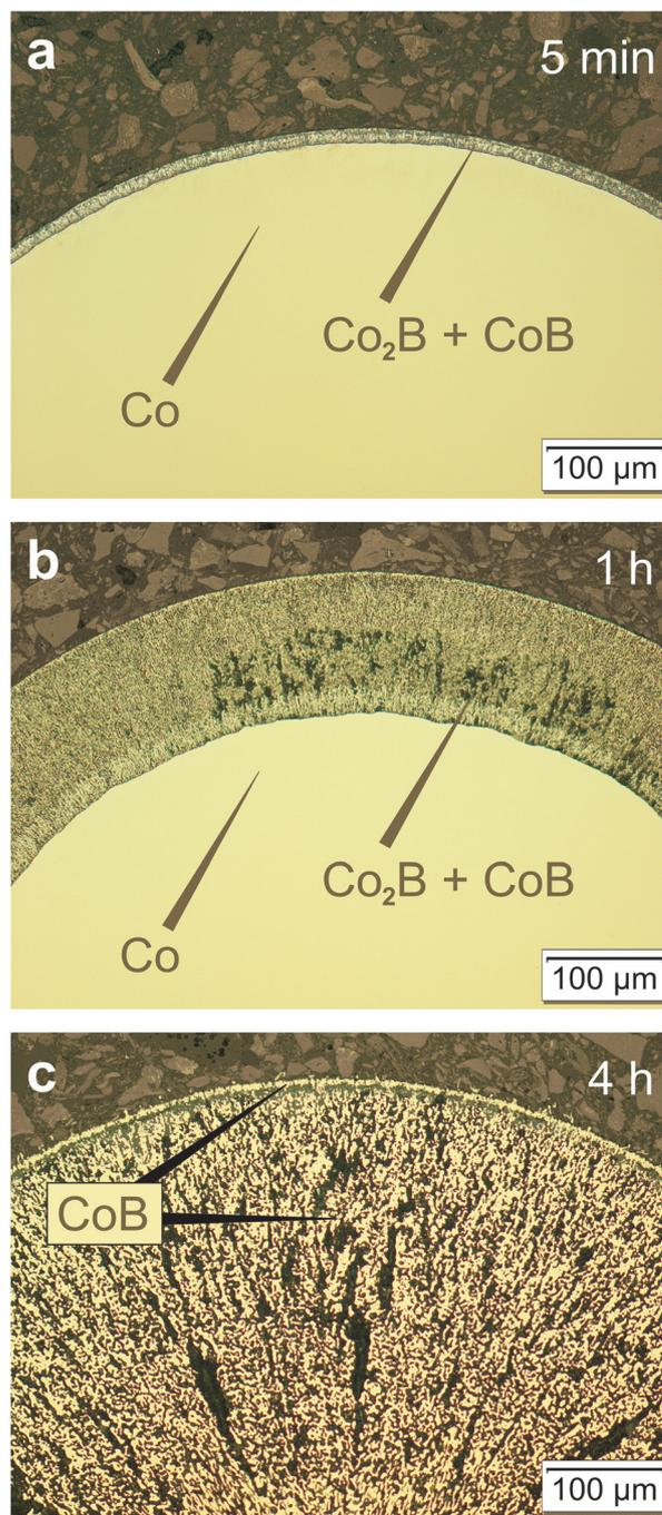
**Fig. 3** Reaction progress between Co(s) and BBr<sub>3</sub>(g) at 700 °C ( $p(\text{BBr}_3) = 94 \text{ mbar}$ ,  $p(\text{Ar}) = 1.9 \text{ mbar}$ ) after 5 min (a), 1 h (b) and 4 h (c). At shorter times (a and b), the Co core is surrounded by two concentric layers of Co<sub>2</sub>B (inner layer) and CoB (outer layer). After the completion of the reaction, the single-phase CoB forms a porous core and a thin, dense surface layer. Optical micrographs (bright field contrast) are shown.
