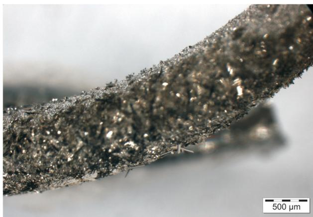
**Fig. 8** The reaction product obtained at 950 °C after 48 h ( $p(\text{BBr}_3) = 94$  mbar,  $p(\text{Ar}) = 190$  mbar). Co<sub>2</sub>B crystals have grown on the surface of the wire. An optical micrograph is shown.
