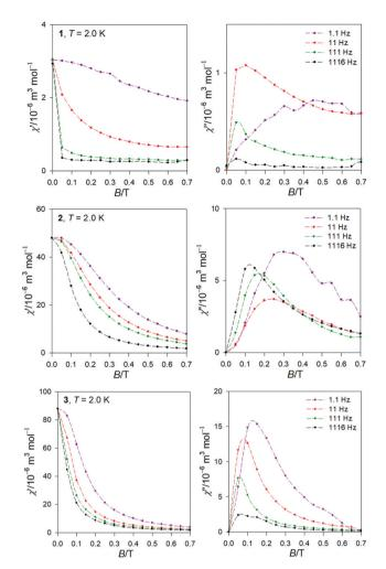
Fig. 5 AC magnetic data for 1, 2, and 3. Field scans for a set of frequencies at low temperature.
