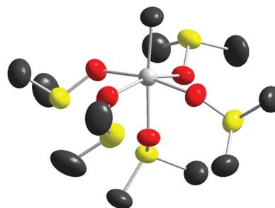
Fig. 1 Structure of the  $[\text{CH}_3\text{Sn}(\text{OS}(\text{CH}_3)_2)_5]^{3+}$  unit in **1**, without a gap. Thermal ellipsoids (at 50% probability) are shown for all atoms; hydrogens have been removed for clarity.
