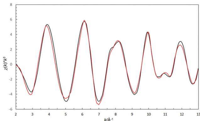
Fig. 2 The almost identical raw EXAFS spectra of solid **1** (red line) and a dmsO solution of **1** (black line) show that the structure of the  $[\text{CH}_3\text{Sn}(\text{OS}(\text{CH}_3)_2)_5]^{3+}$  unit in **1** is maintained in dmsO solution.
