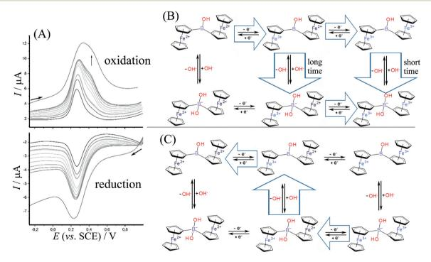
Fig. 4 (A) Redox properties of 1 immobilized in a titanate nanosheet film immersed in aqueous 0.1 M Na₂SO₄. Square wave voltammograms (modulation amplitude 0.02 V, frequency 25 Hz, scan rate 0.12, 0.25, 0.37, 0.4, 0.5, 0.6, 0.7, 0.8, 0.9, 1.0, 2.0 V s<sup>-1</sup>), (B) reaction scheme for oxidation with a short-lived Fe $^{3+}$ /Fe $^{2+}$  species only detected at scan rates higher than 0.4 V s $^{-1}$ . (C) Reaction scheme for reduction via a single reaction pathway.
