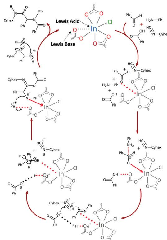
**Fig. 9** Ugi 4-component proposed mechanism for **InPF-51** catalyst.
