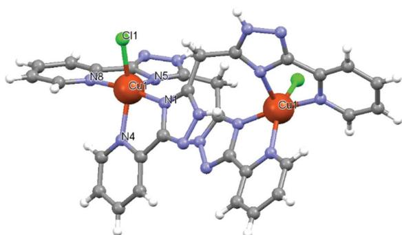
**Fig. 1** Molecular structure of **1**. Counter-anions and solvent molecules are omitted for clarity. Selected bond lengths (in Å): Cu1–N1 1.970(3), Cu1–N8 1.989(3), Cu1–N4 2.091(3), Cu1–N5 2.187(3), and Cu1–Cl1 2.2709.
