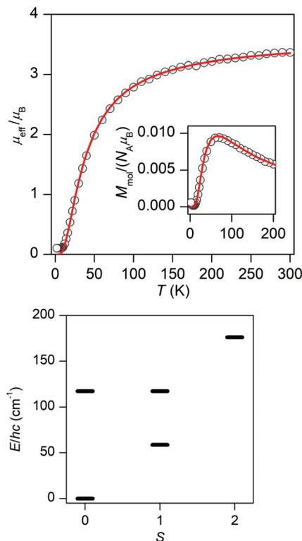
Fig. 6 Top: Temperature dependence of the effective magnetic moment (calculated from magnetization at  $B = 0.5 \text{ T}$ ) of **2** with the low-temperature region expanded in the inset. Circles = experimental points, lines = calculated using the best-fit parameters:  $J = -58.7 \text{ cm}^{-1}$  and  $g = 2.09$ . Bottom: The calculated energy levels according to spin  $S$ .
