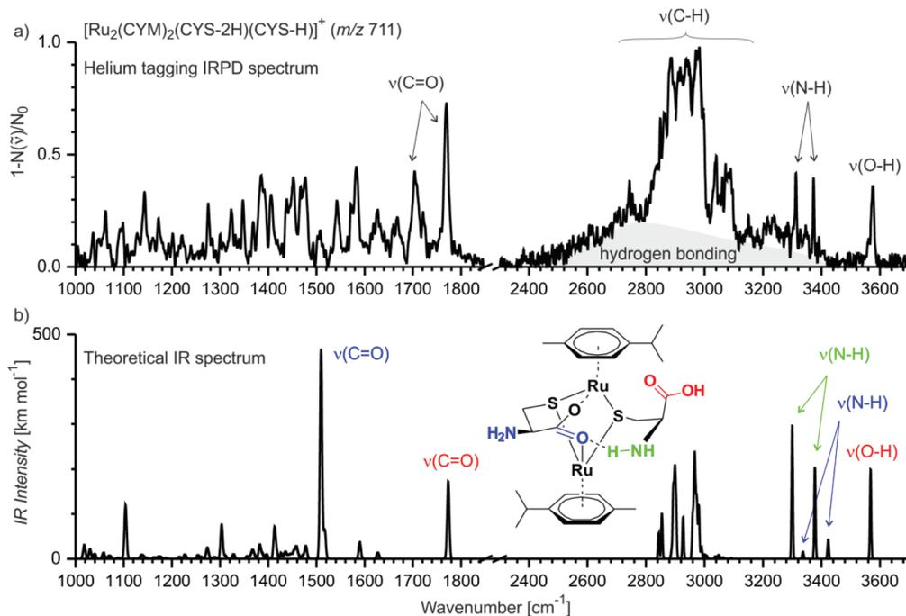
Fig. 7 (a) Helium-tagging IRPD spectrum of mass-selected ion  $[\text{Ru}_2(\text{CYM})_2(\text{Cys-2H})(\text{Cys-H})]^+$  ( $m/z$  711). (b) Theoretical IR spectrum (B3LYP-D3/6-31G\*\*::SDD(Ru)) of one of the possible isomers of  $[\text{Ru}_2(\text{CYM})_2(\text{Cys-2H})(\text{Cys-H})]^+$  (IR spectra of other isomers are shown in Fig. S14,† the xyz coordinates for all reported structures are in the ESI† and can be visualised).
