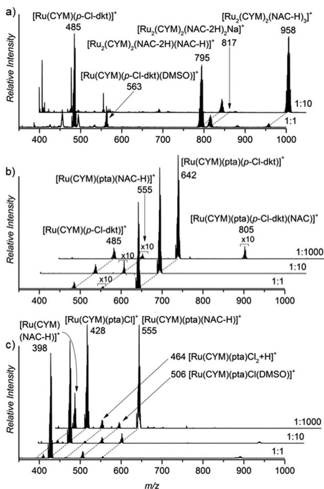
Fig. 2 ESI mass spectra of a 0.2 mM aqueous solution of (a)  $[\text{Ru}(\text{CYM})(p\text{-Cl-dkt})\text{Cl}]$  (b)  $[\text{Ru}(\text{CYM})(\text{pta})(p\text{-Cl-dkt})\text{PF}_6]$  and (c) RAPTA-C with NAC. The spectra were acquired immediately after preparing a solution with all components. The molar ratio of the ruthenium(ii) complex to NAC was 1:1, 1:10 and 1:1000 as denoted in each ESI mass spectrum (right bottom).
