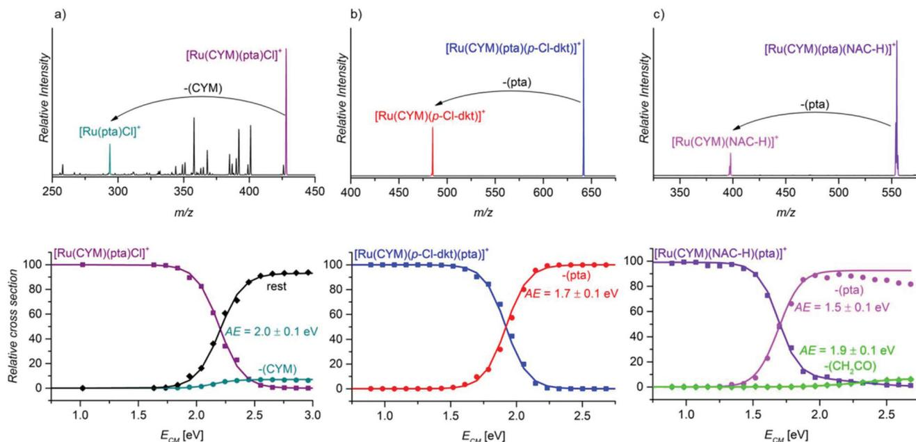
**Fig. 5** (a) The CID spectra of mass-selected ions (a)  $[\text{Ru}(\text{CYM})(\text{pta})\text{Cl}]^+$  ( $E_{\text{coll}}$  2.2 eV at the center of mass frame, c.m.), (b)  $[\text{Ru}(\text{CYM})(\text{pta})(p\text{-Cl-dkt})]^+$  ( $E_{\text{coll}}$  1.8 eV, c.m.) and (c)  $[\text{Ru}(\text{CYM})(\text{pta})(\text{NAC-H})]^+$  ( $E_{\text{coll}}$  1.5 eV, c.m.), and their breakdown curves as function of collision energies.
