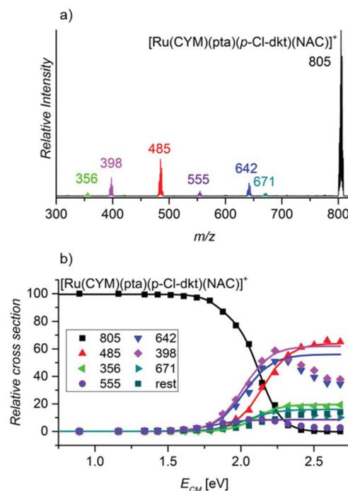
**Fig. 6** (a) The CID spectrum of mass-selected  $[\text{Ru}(\text{CYM})(\text{pta})(p\text{-Cl-dkt})(\text{NAC})]^+$  ( $E_{\text{coll}}$  2.1 eV, c.m.) and (b) breakdown curves. Breakdown curves of the fragments with  $m/z$  671, 642, 555, 398 and 356 were enlarged five times.
