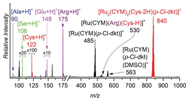
**Fig. 4** ESI mass spectrum of a 0.2 mM aqueous solution of [Ru(CYM)(p-Cl-dkt)]Cl with equimolar concentrations of Cys, Ala, Ser, Glu and Arg. The spectra were acquired immediately after preparing a solution with all components.
