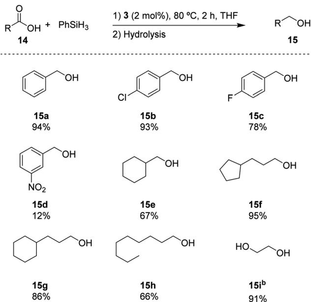
**Scheme 3** Substrate screening for the hydrosilylation of carboxylic acids catalysed by **3**. Reaction conditions: 0.5 mmol substrate, 2 mol% of **3**, 1 mmol of silane, 0.2 mL THF, 80 °C, 2 h. Quantified by  $^1\text{H}$  NMR using mesitylene as an internal standard. <sup>b</sup> 2 mmol of silane.
