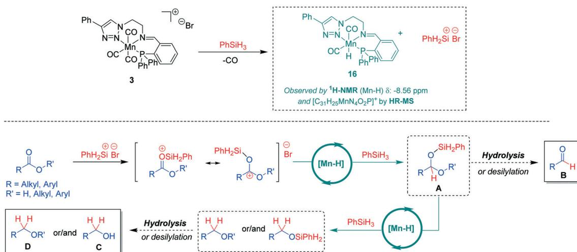
**Scheme 4** A tentative reaction mechanism for Mn(i)-catalysed hydrosilylation of carboxylic groups in acids or esters.
