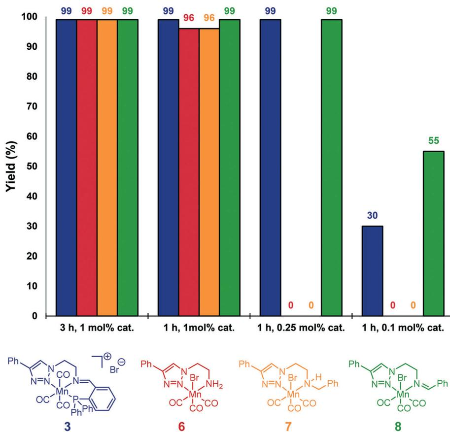
**Fig. 1** Screening of reaction times and Mn(I) complexes for the hydrosilylation of 4a. Reaction conditions: 0.5 mmol acetophenone, 0.5 mmol phenylsilane, 0.2 mL THF, 80 °C. Quantified by <sup>1</sup>H NMR using mesitylene as internal standard.
