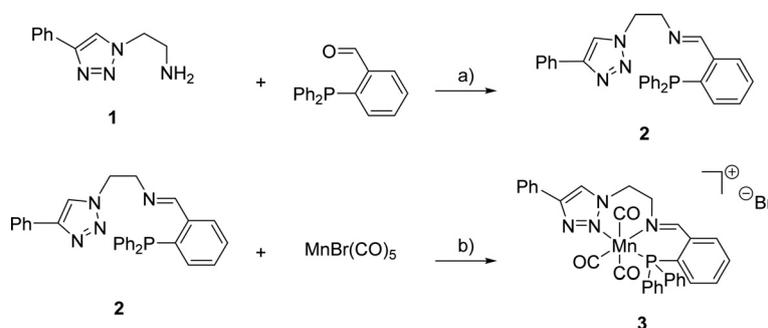
**Scheme 1** Reagents and conditions for the synthesis of **2** and **3**: a) MgSO<sub>4</sub>, toluene, 105 °C, 16 h, 99%; b) toluene, r.t., 60 h, 46%.
