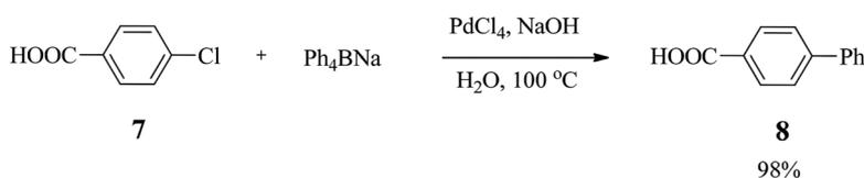
**Scheme 3** Ligand-free Pd-catalysed synthesis of biphenyl-4-carboxylic acid.
