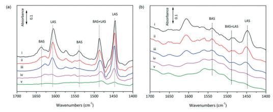
Fig. 4 (a) SnO<sub>2</sub>/Nb<sub>2</sub>O<sub>5</sub>-3.07 and (b) SnO<sub>2</sub>/Nb<sub>2</sub>O<sub>5</sub>-3.07 treated at 500 °C for 1 h, then exposed to water vapor at 150 °C for another 1 h, outgassed at room temperature and subjected to a pyridine adsorption-desorption procedure.
