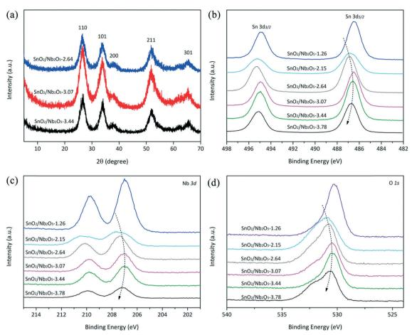
Fig. 2 X-ray diffraction patterns (a) and XPS spectra (b-d) of the SnO<sub>2</sub>/Nb<sub>2</sub>O<sub>5</sub> samples.
