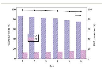
Fig. 8 Results of the reusability study (conditions: [DHA]<sub>o</sub> = 0.2 M,  $SnO_2/Nb_2O_5-3.07 = 50 \text{ mg}, 140 \, ^{\circ}C, 1 \text{ h}).$
