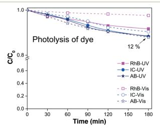
Fig. 1 Variations of the relative concentrations  $C_{\mathrm{photo}}$  of the three dyes due to the photolysis process when the solution is irradiated with visible light (open symbols) and UV light (filled symbols).
