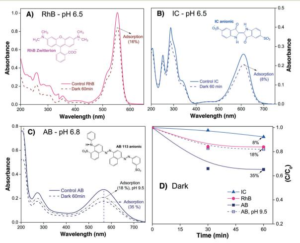
Fig. 2 (A–C) Absorbance spectra of three dye solutions and their evolution after 60 minutes in the dark in the presence of  $\alpha/\beta$ -Bi<sub>2</sub>O<sub>3</sub> powder. D) Variations of  $C_n/C_0$  due to adsorption of the dye molecules on the semiconductor surface in dark conditions; lines are drawn as a visual aid.
