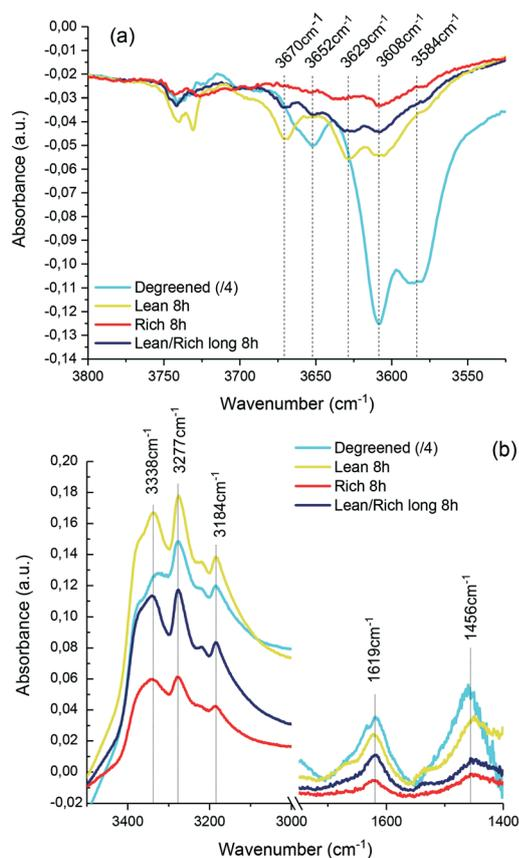
**Fig. 7** DRIFT spectra recorded after 20 min  $\text{NH}_3$  adsorption at 150 °C (1000 ppm  $\text{NH}_3$  in Ar, total flow = 50 mL  $\text{min}^{-1}$ ) and subsequent Ar flushing (55 min) on degreened, rich 8 h, lean 8 h and L/R 8 h aged samples. (a) O–H stretching region and (b) N–H stretching and bending region. The degreened catalyst absorbance was divided by 4.
