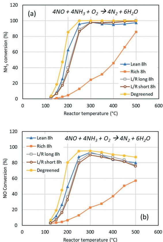
**Fig. 2** Standard SCR activity of degreened and aged Cu/SSZ-13 catalysts. (a)  $\text{NH}_3$  conversion and (b) NO conversion (500 ppm NO, 500 ppm  $\text{NH}_3$ , 8%  $\text{O}_2$ , 5%  $\text{H}_2\text{O}$  in Ar. Total flow =  $3.5 \text{ L min}^{-1}$ ). Aging at  $800^\circ\text{C}$  using lean conditions: 500 ppm NO, 8%  $\text{O}_2$ , 10%  $\text{H}_2\text{O}$  and 10%  $\text{CO}_2$  and rich conditions: 500 ppm NO, 1%  $\text{H}_2$ , 10%  $\text{H}_2\text{O}$  and 10%  $\text{CO}_2$ .
