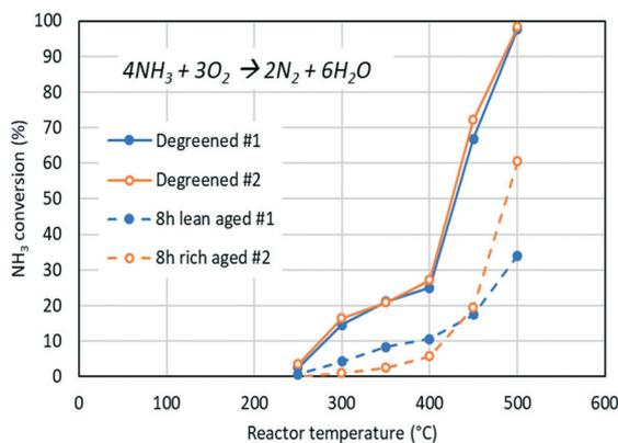
**Fig. 4** NH<sub>3</sub> oxidation activity of degreened and aged Cu/SSZ-13 catalysts. Lean and rich-aged catalysts at all temperatures (500 ppm NH<sub>3</sub>, 8% O<sub>2</sub>, 5% H<sub>2</sub>O in Ar. Total flow = 3.5 L min<sup>-1</sup>). Aging at 800 °C using lean conditions (#1): 500 ppm NO, 8% O<sub>2</sub>, 10% H<sub>2</sub>O and 10% CO<sub>2</sub> and rich conditions (#2): 500 ppm NO, 1% H<sub>2</sub>, 10% H<sub>2</sub>O and 10% CO<sub>2</sub>.
