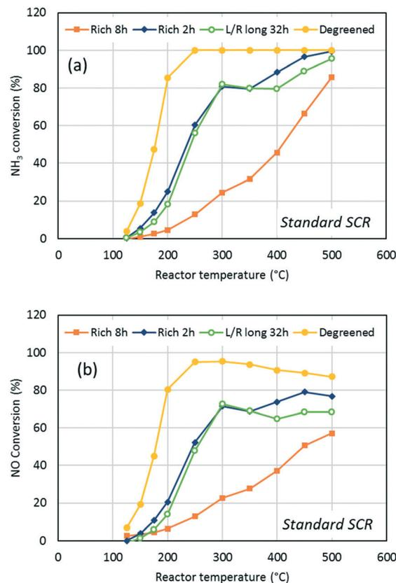
**Fig. 3** Standard SCR activity of degreened and aged Cu/SSZ-13 catalysts. (a)  $\text{NH}_3$  conversion and (b) NO conversion (500 ppm NO, 500 ppm  $\text{NH}_3$ , 8%  $\text{O}_2$ , 5%  $\text{H}_2\text{O}$  in Ar. Total flow =  $3.5 \text{ L min}^{-1}$ ). Aging at  $800^\circ\text{C}$  using lean conditions: 500 ppm NO, 8%  $\text{O}_2$ , 10%  $\text{H}_2\text{O}$  and 10%  $\text{CO}_2$  and rich conditions: 500 ppm NO, 1%  $\text{H}_2$ , 10%  $\text{H}_2\text{O}$  and 10%  $\text{CO}_2$ .
