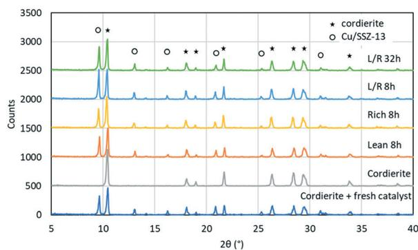
**Fig. 1** X-ray diffractogram of a mixture of fresh Cu/SSZ-13 (25 wt%) + cordierite (75 wt%), pure cordierite and crushed monolithic samples after aging for 8 h in lean (lean 8 h), 8 h in rich (rich 8 h), 8 h in cycling conditions between lean (15 min) and rich (1 min) (L/R 8 h) and 32 h in cycling conditions between lean (15 min) and rich (1 min) (L/R 32 h).
