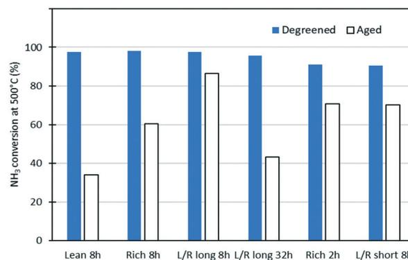
**Fig. 5** NH<sub>3</sub> oxidation activity of degreened and aged Cu/SSZ-13 catalysts. All catalysts at 500 °C (500 ppm NH<sub>3</sub>, 8% O<sub>2</sub>, 5% H<sub>2</sub>O in Ar. Total flow = 3.5 L min<sup>-1</sup>). Aging at 800 °C using lean conditions: 500 ppm NO, 8% O<sub>2</sub>, 10% H<sub>2</sub>O and 10% CO<sub>2</sub> and rich conditions: 500 ppm NO, 1% H<sub>2</sub>, 10% H<sub>2</sub>O and 10% CO<sub>2</sub>.
