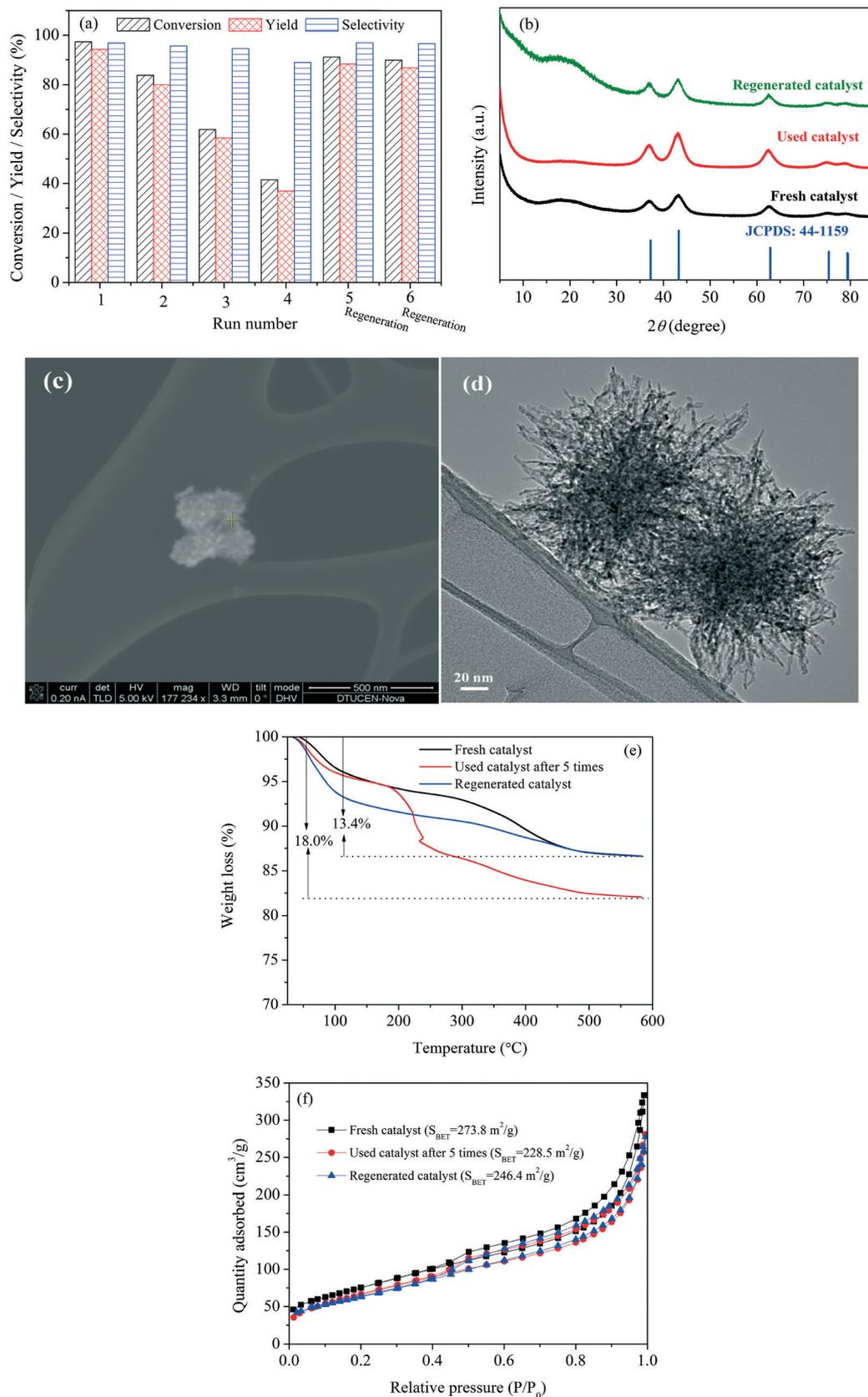
**Fig. 5** (a) Catalytic performance of NiO(P)-300 in the CTH of FF to FAOL during recycling. (b) XRD patterns of fresh, used and regenerated NiO(P)-300 catalysts. (c) SEM image of used NiO(P)-300 catalyst. (d) TEM image of used NiO(P)-300 catalyst. (e) TG curves of fresh, used and regenerated NiO(P)-300 catalysts. (f)  $N_2$  adsorption-desorption isotherms of fresh, used and regenerated NiO(P)-300 catalysts. Reaction conditions: 1 mmol FF, 0.02 g NiO(P)-300, 5 mL 2-propanol, 120 °C, 3 h.
