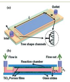
Fig. 9 Schematic of a typical microfluidic device with multiple channels in a tree like distribution. Image reproduced from ref. 53 with permission from The Royal Society of Chemistry.
