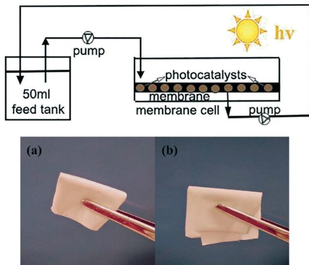
Fig. 11 Schematic of the recirculation membrane photoreactor system used by Yu *et al.* and the flexibility of the polymeric membrane used. Reprinted from ref. 59, copyright 2018, with permission from Elsevier.
