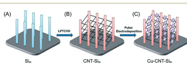
**Fig. 6** Schematic representation of the fabrication process including electrodeposition of suspended CuO on CNT fibres. Image reproduced from ref. 43 with permission from The Royal Society of Chemistry.
