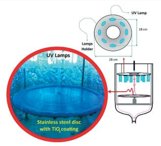
Fig. 10 Jet impinging of a pollutant solution onto a TiO<sub>2</sub> coated disk surface in the set up. Reprinted from ref. 57, copyright 2017, with permission from Elsevier.
