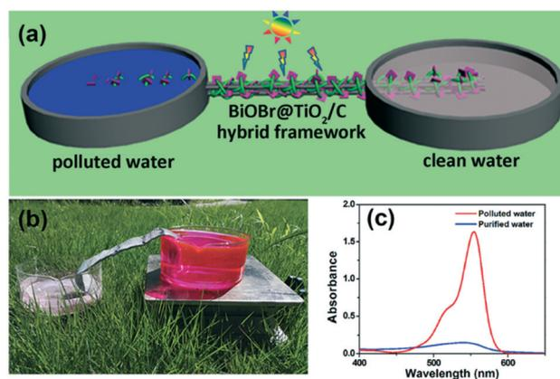
Fig. 14 (a) Schematic image of the un-powered flow reactor used by Mei *et al.* (b) Photograph of the system in operation under solar irradiation and (c) the removal of rhodamine B using the system. Image reproduced from ref. 64 with permission from The Royal Society of Chemistry.
