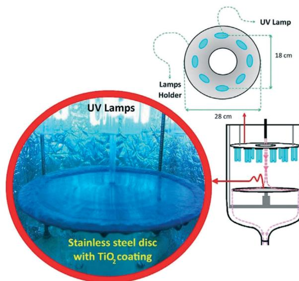
Fig. 10 Jet impinging of a pollutant solution onto a TiO<sub>2</sub> coated disk surface in the set up. Reprinted from ref. 57, copyright 2017, with permission from Elsevier.
