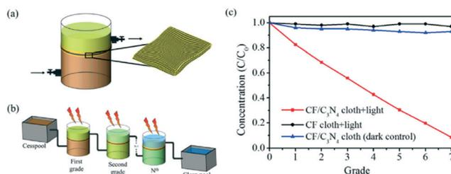
Fig. 12 Photocatalytic membrane system devised by Shen *et al.* showing (a) a single grade system where pollutant is pumped through the membrane, (b) the connection of several grade systems in series and (c) the improvement in Rhodamine B removal after multiple degradation grades. Reprinted from ref. 60, copyright 2017, with permission from Elsevier.
