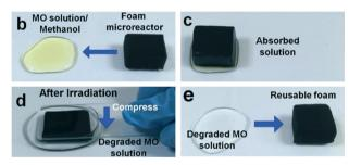
Fig. 13 Uptake of MO solution by soaking of the foam microreactor developed by Zhu et al. and subsequent regeneration of the foam leaving the purified solution. Reprinted from ref. 63, copyright 2015, with permission from Wiley-VCH.
