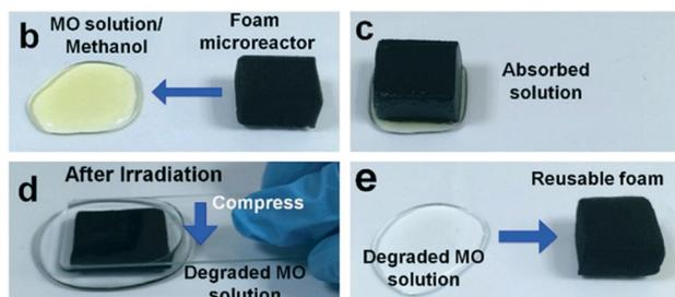
Fig. 13 Uptake of MO solution by soaking of the foam microreactor developed by Zhu *et al.* and subsequent regeneration of the foam leaving the purified solution. Reprinted from ref. 63, copyright 2015, with permission from Wiley-VCH.
