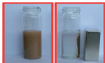
Fig. 2 Magnetic separation of a magnetic nanocomposite post use. Image reproduced from ref. 24 with permission from The Royal Society of Chemistry.
