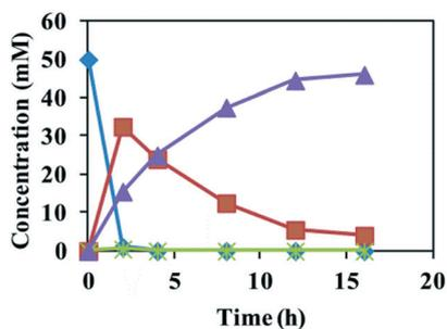
**Fig. 1** Time course of the conversion of styrene oxide **1c** (50 mM) to (*S*)-**4c** with resting cells of *E. coli* (SpEH-BDHA-GoSCR-MVTA) (20 g cdw L<sup>-1</sup>) in a two-liquid phase system. ◆ = the concentration of **1c**; ■ = the concentration of **2c**; ✕ = the concentration of **3c**; and ▲ = the concentration of (*S*)-**4c**.
