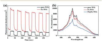
Fig. 8 (a) Photocurrent curves of pure WO<sub>3</sub> and 0.25 mol% Fe-doped WO<sub>3</sub>; (b) PL spectra of pure WO<sub>3</sub>, 0.25 mol% Fe-doped WO<sub>3</sub> and 0.75 wt% Pt@0.25 mol% Fe-WO3.
