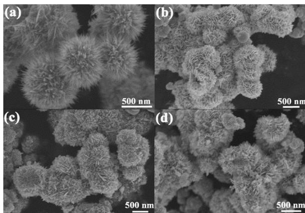
Fig. 4 SEM images of (a) bare  $\text{WO}_{2.72}$ , (b) pure  $\text{WO}_3$  ( $\text{WO}_{2.72}$  calcined at  $450\text{ }^\circ\text{C}$  for 1.5 h), (c) 0.25 mol% Fe-doped  $\text{WO}_3$  (0.25 mol% Fe-doped  $\text{WO}_{2.72}$  calcined at  $450\text{ }^\circ\text{C}$  for 1.5 h), (d) 0.75 wt% Pt@0.25 mol% Fe- $\text{WO}_3$  after 9 time photocatalytic degradation experiments.
