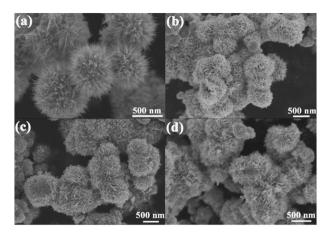
Fig. 4 SEM images of (a) bare WO<sub>2.72</sub>, (b) pure WO<sub>3</sub> (WO<sub>2.72</sub> calcined at 450 °C for 1.5 h), (c) 0.25 mol% Fe-doped WO $_3$  (0.25 mol% Fedoped WO<sub>2.72</sub> calcined at 450 °C for 1.5 h), (d) 0.75 wt% Pt@0.25 mol% Fe-WO<sub>3</sub> after 9 time photocatalytic degradation experiments.
