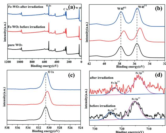
Fig. 6 (a) XPS survey spectra and (b and c) high-resolution XPS spectra of W 4f and O 1s for pure  $\text{WO}_3$  and 0.25 mol% Fe-doped  $\text{WO}_3$  before and after irradiation, (d) high-resolution XPS spectra of Fe 2p for 0.25 mol% Fe-doped  $\text{WO}_3$  before and after irradiation.
