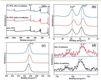
Fig. 6 (a) XPS survey spectra and (b and c) high-resolution XPS spectra of W 4f and O 1s for pure  $WO_3$  and 0.25 mol% Fe-doped  $WO_3$  before and after irradiation, (d) high-resolution XPS spectra of Fe 2p for 0.25 mol% Fe-doped WO<sub>3</sub> before and after irradiation.
