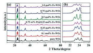
Fig. 2 The XRD spectra (a) and the enlarged XRD spectra (b) of the pure WO<sub>3</sub>, Fe-doped WO<sub>3</sub> and Pt@Fe-WO<sub>3</sub> samples.
