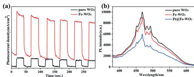
Fig. 8 (a) Photocurrent curves of pure  $\text{WO}_3$  and 0.25 mol%  $\text{Fe-doped WO}_3$ ; (b) PL spectra of pure  $\text{WO}_3$ , 0.25 mol%  $\text{Fe-doped WO}_3$  and 0.75 wt%  $\text{Pt@0.25 mol\% Fe-WO}_3$ .
