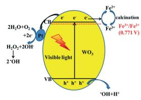
Fig. 9 Proposed schematic diagram of charge transfer in the Pt@Fe-WO<sub>3</sub> system under visible-light irradiation.
