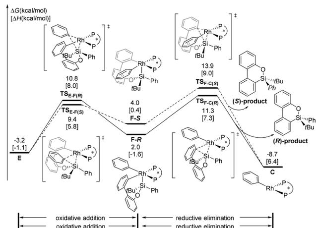
Fig. 4 The free energy profiles for the oxidative addition and reductive elimination mechanisms.
