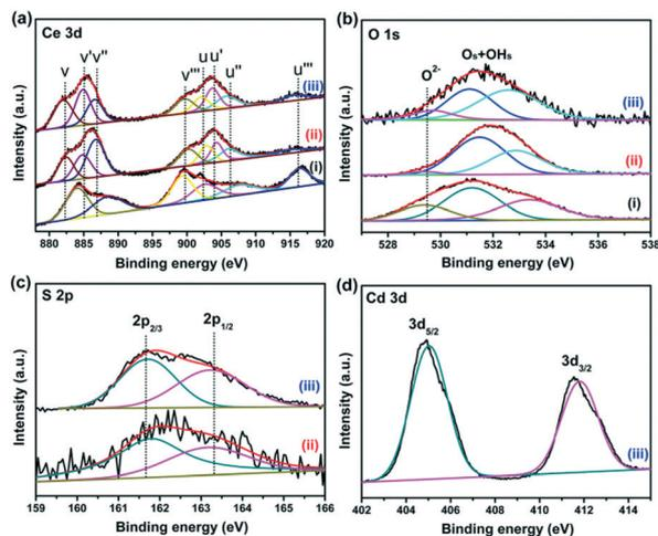
Fig. 3 High-resolution XPS spectra of (a) Ce 3d, (b) O 1s, (c) S 2p and (d) Cd 3d; (i), (ii) and (iii) represent  $\text{CeO}_2$ ,  $\text{CeO}_{2-x}\text{S}_x$ , and  $\text{CeO}_{2-x}\text{S}_x@\text{CdS}$ , respectively.
