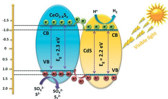
**Scheme 2** Schematic diagram of the proposed charge carrier transfer and H<sub>2</sub> evolution mechanism over the CeO<sub>2-x</sub>S<sub>x</sub>@CdS photocatalyst under visible-light irradiation.
