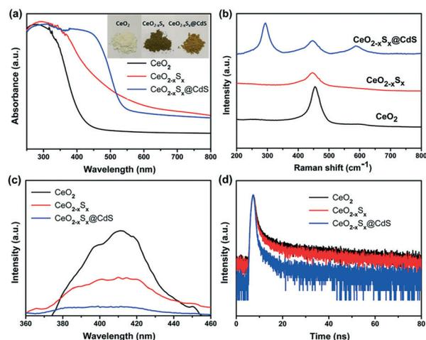
Fig. 4 (a) UV-visible diffuse reflectance absorption spectra, (b) Raman spectra, (c) photoluminescence spectra, and (d) TRPL spectra of the  $\text{CeO}_2$ ,  $\text{CeO}_{2-x}\text{S}_x$  and  $\text{CeO}_{2-x}\text{S}_x@\text{CdS}$  samples.
