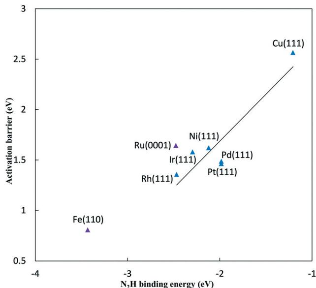
**Fig. 3** Activation barriers for  $\text{N}_2$  to  $\text{N}_2\text{H}^*$  reduction on late transition metal surfaces at 0 V-RHE, plotted against  $\text{N}_2\text{H}^*$  binding energy to the same surface. Blue – FCC(111) metal surfaces, purple – Fe(110) and Ru(0001) surfaces. Linear best fit are shown for FCC metals,  $G_{a1} = 0.93$  ( $\text{N}_2\text{H}$  binding energy) + 3.55 eV ( $R^2 = 0.83$ ).
