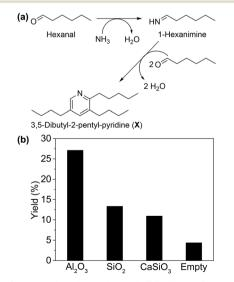
Fig. 1 (a) Scheme for formation of 3,5-dibutyl-2-pentyl-pyridine (compound X) and (b) yield of compound X with different supports. Reaction conditions: 1 μL min<sup>-1</sup> hexanal, 200 mg catalyst, 190 °C, 8 mL  $min^{-1} NH_3$ , 20 mL  $min^{-1} N_2$ . GHSV = 1.12 × 10<sup>4</sup>  $h^{-1}$ .
