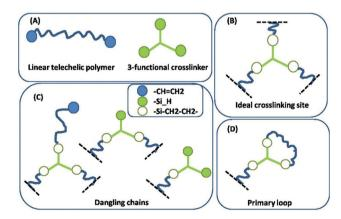
Some common first order imperfections in networks. (A) The two constituents in the network (reactants). (B) An ideal, elastic junction. The black dashed lines indicate connections to the infinite network. (C) Dangling chains of first order, i.e. dangling structures, which consist solely of one of each constituent or a set thereof. (D) A primary inelastic loop. Reproduced from ref. 14 with permission from the Technical University of Denmark (DTU), copyright 2017.
