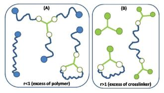
Fig. 5 Illustration of the most common sol structures for the two scenarios of (A) excess of polymer and (B) excess crosslinker. Networks resulting from r < 1 possess by far the most complex dynamical behaviour, whereas those resulting from r > 1 may be prone to curing over time when the utilised crosslinker is hydride-functional. Reproduced from ref. 14 with permission from the Technical University of Denmark (DTU), copyright 2017.
