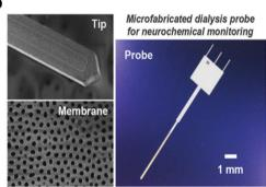
Fig. 10 Neural devices for chemical monitoring. (a) Multi-electrode micro-needle for in vivo neurochemical monitoring. Reproduced with permission from ref. 204. Copyright 2015 Elsevier. (b) Microdialysis probe for neurochemical monitoring. Reproduced with permission from ref. 209. Copyright 2016 American Chemical Society.
