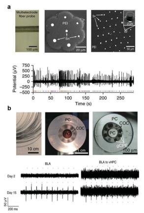
Fig. 20 Flexible and multifunctional fiber probes. (a) Multielectrode PEI/ Sn fiber probe to record spontaneous single-neuron activity. Reproduced with permission from ref. 70. Copyright 2015 Nature Publishing Group. (b) Multifunctional probes with PC/COC/gCPE combination for one-step optogenetics. Reproduced with permission from ref. 71. Copyright 2017 Nature Publishing Group.
