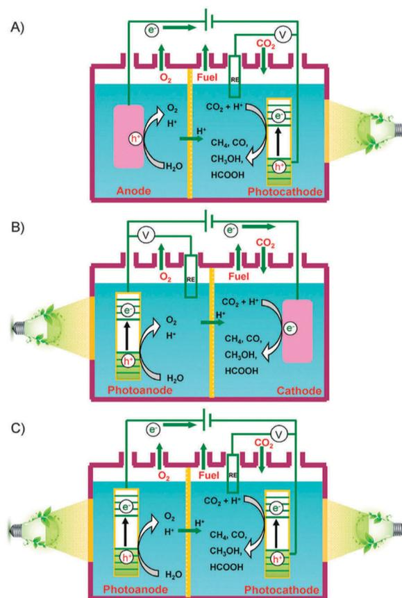
Fig. 35 Schematic representation of photoelectrocatalytic reactors in two-compartment cells separated by proton-exchange membranes. CO<sub>2</sub>RR and water oxidation occur over the cathode and the anode sides, respectively. The alternative or simultaneous utilization of photocatalysts under light irradiation on the cathode and anode side is represented in each case. Reprinted with permission from ref. 539. Copyright The Royal Society of Chemistry 2016.
