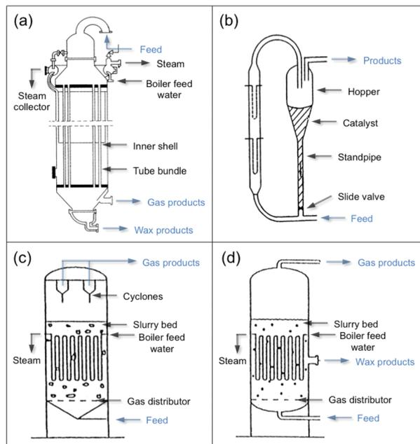
**Fig. 14** Schematic representations of (a) a multi-tubular fixed bed reactor and (b–d) three types of fluidized bed reactors: (b) circulating fluidized bed, (c) ebullated or fixed fluidized bed, and (d) slurry phase bubbling bed. Types (b) and (c) are two-phase systems. In type (d),  $\text{CO}_2$  and  $\text{H}_2$  pass through a liquid in which the solid catalyst particles are suspended. Adapted with permission from ref. 216. Copyright 2002 Elsevier B.V.
