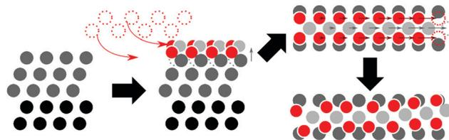
Fig. 2 Initial geometry production process, from left to right: (side view) surface optimization, formation of full coverage  $\text{PtO}_2$  stripe by lifting one surface row, (top view) omission of one  $\text{PtO}_2$  unit from an  $\text{PtO}_2$  covered surface supercell, and rearrangement of Pt and O atoms (illustrating final structure after both initial manual displacement/dilation and DFT geometry relaxation).
