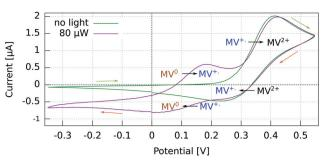
Fig. 4 Cyclic voltammogram in the dark and under light at 830 nm of a p-GaAs electrode vs. Pt using a 2 mM MV $^{+\bullet}$  solution in acetonitrile with 200 mM TBAP. Recorded at 50 mV s $^{-1}$  with a Pt rod CE.
