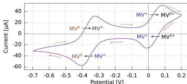
Fig. 3 Cyclic voltammogram for GaN/Au/Al(5)/Ag WE vs. Pt using a 2 mM  $MV^{+\bullet}$  solution in acetonitrile with 200 mM TBAP. Recorded at 50  $\text{mV s}^{-1}$  with a Pt rod CE. Reactions indicated in the sense of the scanning direction.
