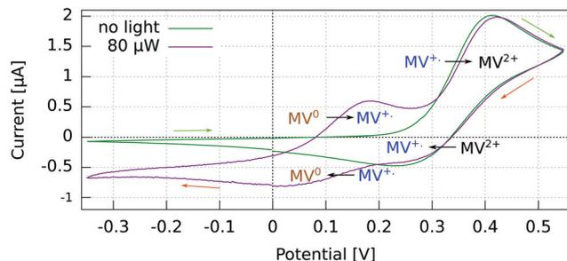
Fig. 4 Cyclic voltammogram in the dark and under light at 830 nm of a p-GaAs electrode vs. Pt using a 2 mM  $MV^{+\bullet}$  solution in acetonitrile with 200 mM TBAP. Recorded at  $50 \text{ mV s}^{-1}$  with a Pt rod CE.
