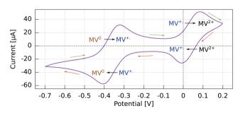
Fig. 3 Cyclic voltammogram for GaN/Au/Al(5)/Ag WE vs. Pt using a 2 mM MV++ solution in acetonitrile with 200 mM TBAP. Recorded at 50 mV s<sup>-1</sup> with a Pt rod CE. Reactions indicated in the sense of the
