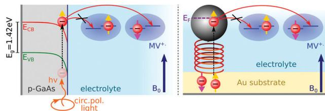
Fig. 1 Principle of the experiment: methyl viologen radicals ( $MV^{+•}$ ) in solution are spin-polarized by a magnetic induction field  $B_0$ . Electrons are transferred from a p-GaAs electrode spin pumped with circularly polarized light (left illustration), or from an Au electrode functionalized with chiral molecules (right illustration).
