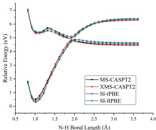
Fig. 5 PESs for N–H bond fission of staggered methylamine with various methods. The relative energies are compared with those of the equilibrium geometry for each method.
