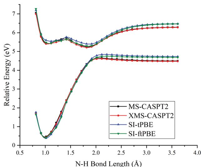
Fig. 8 PESs for N–H bond fission of methylamine with H6–C4–N1–H3 dihedral angle equaling 100° using various methods. The relative energies are compared with those of the equilibrium geometry for each method.
