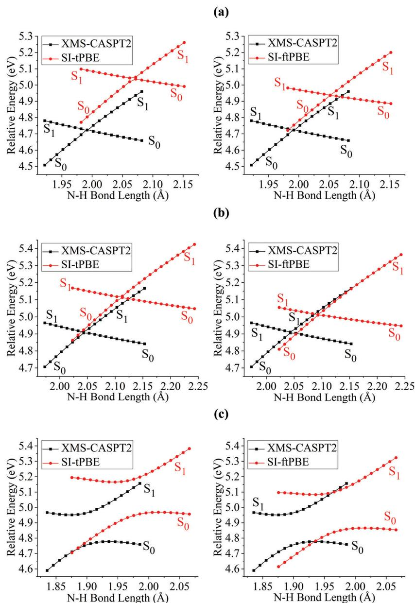
**Fig. 6** PESs for N–H bond fission of (a) eclipsed-H3, (b) eclipsed-H2 and (c) staggered methylamine near the LAC region with various methods. The relative energies are compared with those of the equilibrium geometry for each method.
