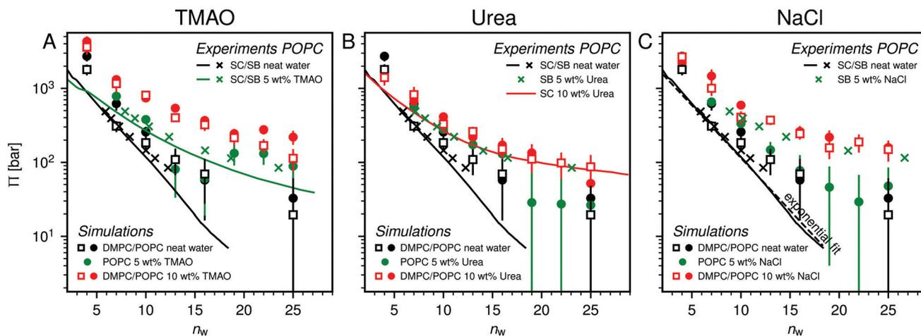
Fig. 2 Pressure–hydration curves  $\Pi(n_w)$  of POPC membranes with and without added TMAO (A), urea (B), and NaCl (C), as obtained in sorption balance (SB – crosses) and sorption calorimetry (SC – solid lines) experiments and simulations. The figure also contains simulation data for DMPC. The dashed line in panel (C) indicates an exponential fit to the sorption calorimetry data in the absence of co-solutes, with decay length  $\lambda_{POPC} = 0.29 \text{ nm}$  (see main text).
