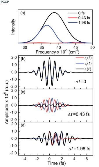
Fig. 3 (a) Spectral profile  $\left|\tilde{\mathscr{E}}(\omega)\right|^2$  (eqn (7)) of the laser field applied with three different time delays between the two Gaussian pulses,  $\Delta t=0$ , 0.43, and 1.98 fs, and temporal profiles of the two Gaussian pulses  $\mathscr{E}_1(t)$  and  $\mathscr{E}_2(t)$  along with their sum  $\mathscr{E}(t)$  for the time delays (b)  $\Delta t=0$ , (c)  $\Delta t=0.43$  fs, and (d)  $\Delta t=1.98$  fs.
