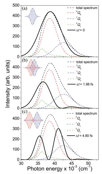
Fig. 2 Calculated absorption spectrum of the A-band of CH<sub>3</sub>I, along with the sub-bands associated with the transitions  ${}^3Q_0 \leftarrow \tilde{X}^1A_1$ ,  ${}^1Q_1 \leftarrow \tilde{X}^1A_1$ , and  ${}^3Q_1 \leftarrow \tilde{X}^1A_1$ . Also shown are the spectral profiles  $\left|\tilde{\mathscr{E}}(\omega)\right|^2$  (eqn (7)) of the laser field of eqn (3) applied with three different time delays, (a)  $\Delta t=0$ , (b) 1.98, and (c) 4.80 fs.
