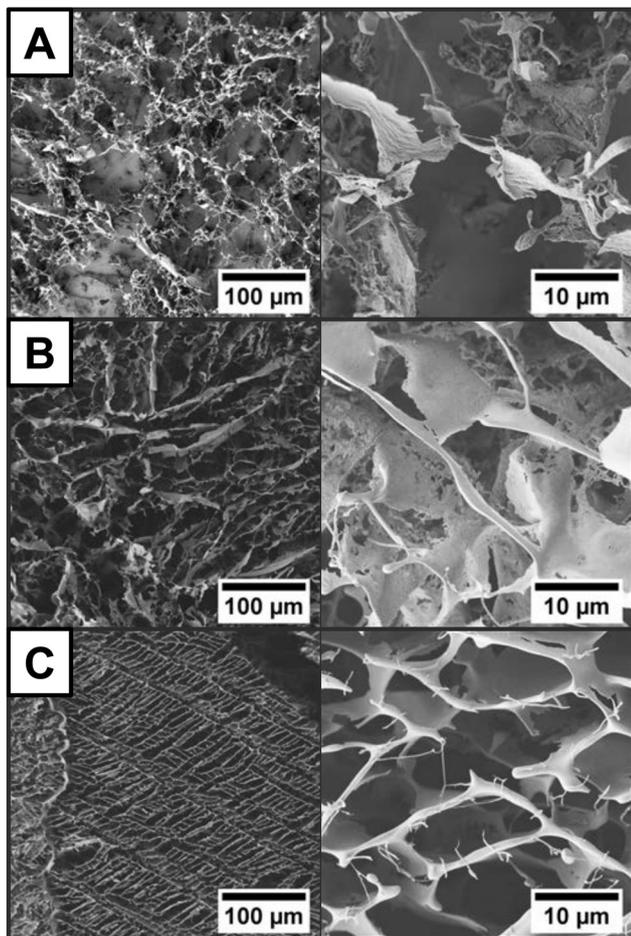
Fig. 3 SEM images of different CdSe NPL cryoaerogel coatings. The concentration of Cd<sup>2+</sup> in the original aqueous NPL solutions increases from panel A to C (A: 10 mM, B: 28 mM, and C: 70 mM). For the preparation of each sample, 20  $\mu$ L of the respective NPL solution was used. The KOH concentration was kept constant at  $1 \times 10^{-2}$  M.
