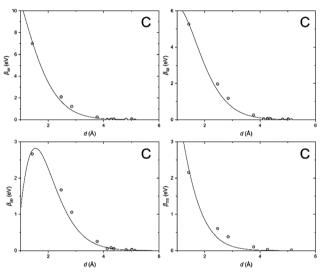
Fig. 6 Distance dependence of the resonance integrals for carbon as obtained by LOBSTER and fitted as being proportional to the overlap integrals.
