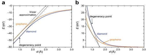
Fig. 3 Energy contributions of diamond and graphene structures of carbon as a function of the interatomic distances: (a) bonding energies of allotropes, (b) core-core repulsion. In (a) and (b), the linear approximation around the degeneracy point has been included (black lines).
