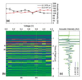
Fig. 5 Raw data colourmap (corresponding to the smoothed data shown in Fig. 4) of the acoustic intensity for a single position (b) with (a) a quantification of the changes in manitude of the acoustic signal for two times-of-flight located at (i) 1.979 µs and (ii) 2.437 µs and (c) time-of-flight investigated at two voltages (iii) 3.4 V and (iv) 3.8 V associated with the charging process for a position 6 in the battery.
