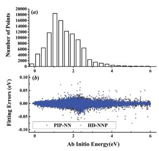
Fig. 3 (a) The distribution of the sampled points, and (b) PIP-NN and HD-NNP fitting errors (eV) as a function of the ab initio energy (eV) relative to the reactant asymptote for the H + NH<sub>3</sub> system.
