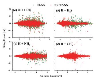
Fig. 7 NRPIP-NN and FI-NN fitting errors (eV) as a function of the ab initio energy (eV) relative to the reactant asymptote for OH + CO (a),  $H + H_2S$  (b) and H + NH<sub>3</sub> (c), respectively, and NRPIP-NN fitting errors (eV) for H + CH<sub>4</sub> (d).
