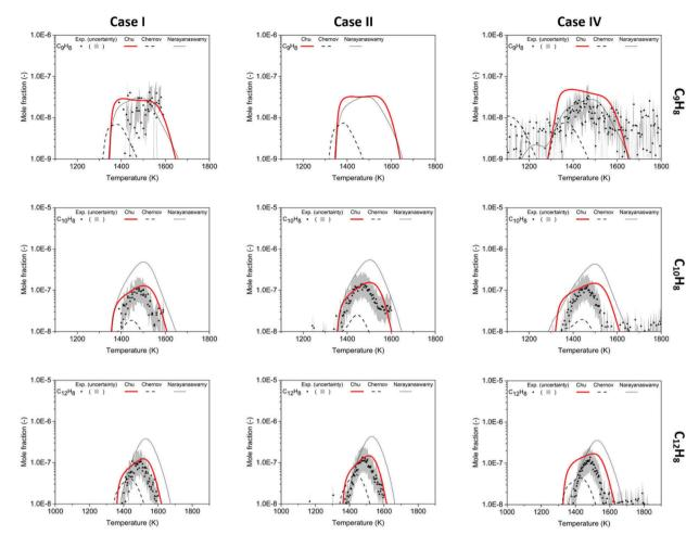
Fig. 7 Mole fraction profiles of  $C_9H_8$ ,  $C_{10}H_8$ ,  $C_{12}H_8$  as a function of oven temperature for Case I, II and IV, measurements (symbols and uncertainty band) and predictions of three models (lines). In the Case II experiment, the  $C_9H_8$  signal was hard to discern above the noise
