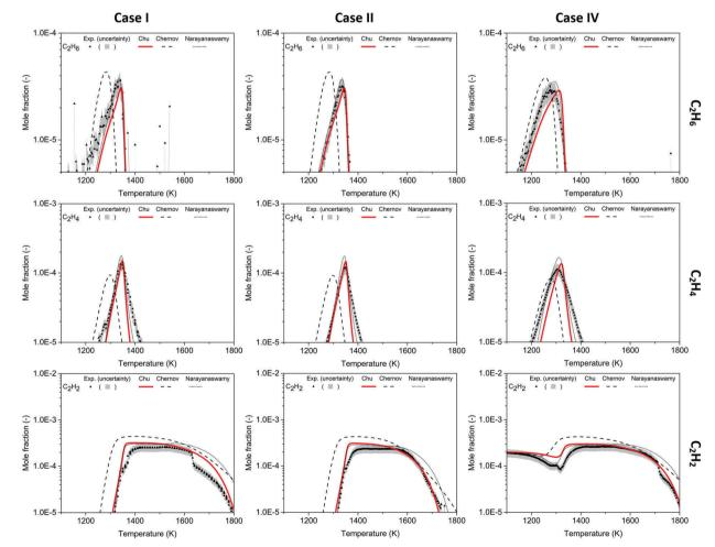
Fig. 3 Mole fraction profiles of C<sub>2</sub>H<sub>6</sub>, C<sub>2</sub>H<sub>4</sub>, C<sub>2</sub>H<sub>2</sub> as a function of oven temperature for Case I, II and IV, measurements (symbols and uncertainty band) and predictions of three models (lines)
