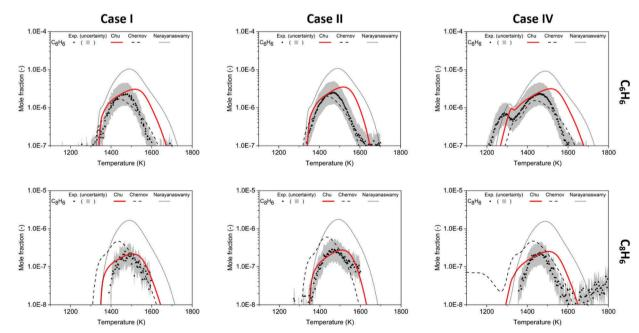
Fig. 6 Mole fraction profiles of C<sub>6</sub>H<sub>6</sub> and C<sub>8</sub>H<sub>6</sub> as a function of oven temperature for Case I, II and IV, measurements (symbols) and model predictions (lines). The gray band indicates experimental uncertainty
