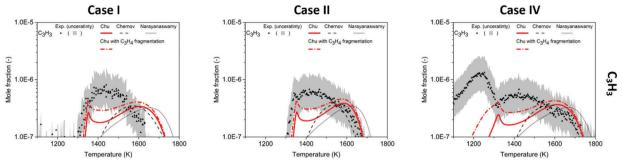
Fig. 5 Mole fraction profiles of  $C_3H_3$  and total m/z = 39 signal as a function of oven temperature for Case I, II and IV, measurements (symbols and uncertainty band) and predictions of three models (lines). Contribution of m/z = 39 fragments from  $C_3H_4$  species are additionally shown and significantly improves the model predictions at lower temperatures.
