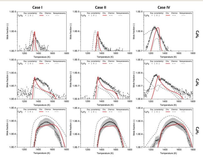
Fig. 4 Mole fraction profiles of C<sub>4</sub>H<sub>6</sub>, C<sub>4</sub>H<sub>4</sub>, C<sub>4</sub>H<sub>2</sub> as a function of oven temperature for Case I, II and IV, measurements (symbols and uncertainty band) and predictions of three models (lines)
