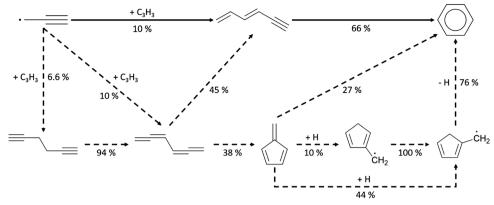
Scheme 3 Leading pathways of benzene formation from propargyl radicals found in the Chu mechanism, and the ROP analysis at the oven temperature (1517 K) maximizing C<sub>6</sub>H<sub>6</sub> concentration in Case 1 (major pathway – solid line, minor pathways – dash line)
