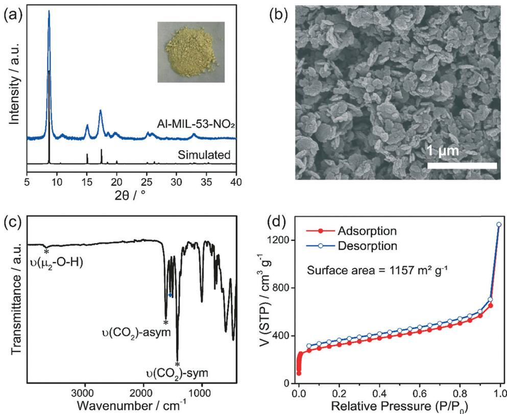
Fig. 1 (a) PXRD patterns and digital image (inset), (b) SEM image, (c) FT-IR spectrum, and (d) gas sorption isotherms of the Al-MIL-53-NO<sub>2</sub> nanoparticles.
