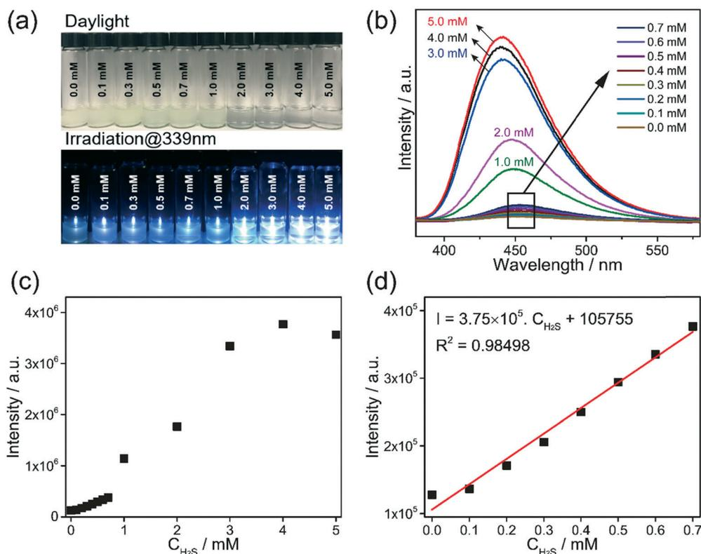
Fig. 2 (a) Digital images of Al-MIL-53-NO<sub>2</sub> suspensions with various NaHS concentrations under visible light (up) and UV light (339 nm, down); (b) emission spectra of Al-MIL-53-NO<sub>2</sub> suspensions with various NaHS concentrations (excitation wavelength: 339 nm); (c and d) emission intensity versus NaHS concentration.
