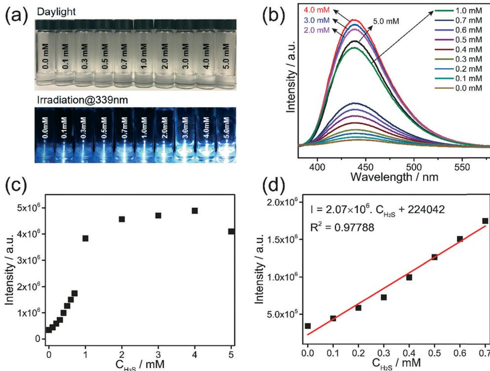
**Fig. 6** (a) Digital images of Al-MIL-53-NO<sub>2</sub> supernatants separated from Al-MIL-53-NO<sub>2</sub> suspensions with various NaHS concentrations under visible light (up) and UV light (339 nm, down); (b) emission spectra of Al-MIL-53-NO<sub>2</sub> supernatants from Al-MIL-53-NO<sub>2</sub> supernatants with various NaHS concentrations (excitation wavelength: 339 nm); (c) and (d) emission intensity versus NaHS concentration.
