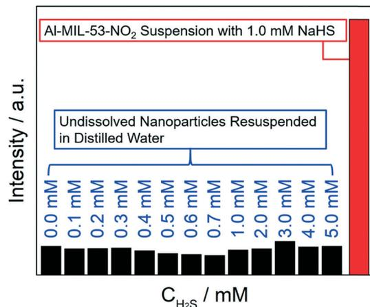
**Fig. 5** Emission intensities at 450 nm (excitation wavelength: 339 nm) of aqueous solutions of undissolved nanoparticles (treated with 0.0 mM to 5.0 mM H<sub>2</sub>S) (black columns) and Al-MIL-53-NO<sub>2</sub> suspension with 1.0 mM NaHS (red column).
